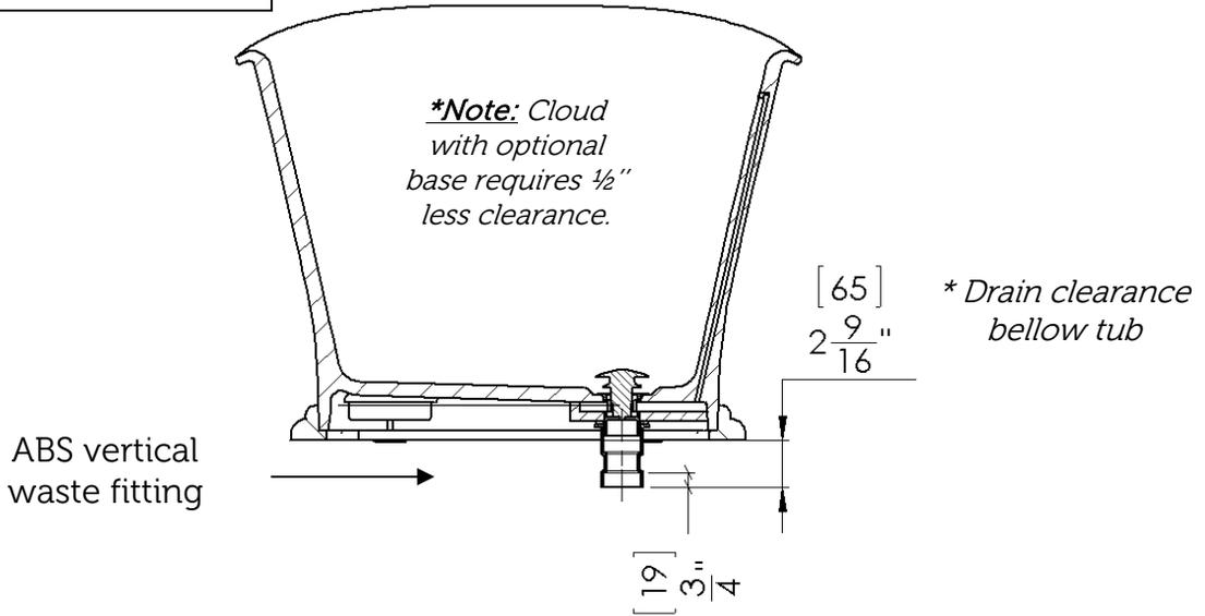
\*\*\* These tub models require vertical plumbing connection from the floor.
